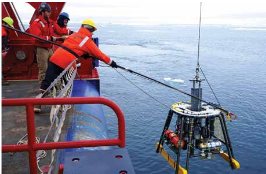
This device, known as a multi-corer, gathers mud samples from the seafloor for analysis in the lab. (Photo: Kim Kenny)
